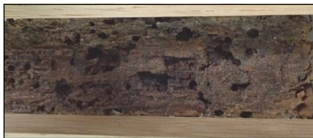
The back of the panel, as with all the panels, is severely degraded. Consolidant was applied in multiple applications over several weeks. The addition of inert fillers will have provided additional support to voids in the wood. However many weak passages could not be accessed. The tracery overlay and the specially designed architectural frame will provide the best protection for the panels once they have been re-installed in the church.
